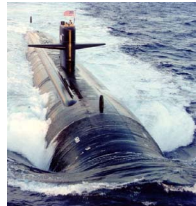
Laminar flow shown at front---- Turbulent flow to the sides. Picture sourced from wikipedia.com
